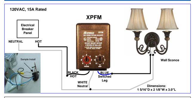
**Description:** The XPFM Fixture Module (Non-Dimming) is designed to control a Load of up to 15A. The XPFM is small enough to fit inside recessed lighting cans and single gang boxes of new or existing lighting fixtures. This allows hard-wired switching control from inside a lighting fixture. Responds to On/Off and ALL LIGHTS ON/ALL UNITS OFF commands. NON Dimming.
